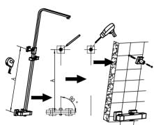
5.Measure the installation height of the shower rail as per dimension A, using a tape measure and spirit level, ensuring that when the top section of the rail which is height adjustable is extended, it can achieve the required height for the users.Mark one hole in required position with pen.Drill the hole in the wall with electric drill and place the wall plug into the hole.Always check before drilling that no cables or pipes can be damaged. Fit the connector to the fixing plate and cover.
